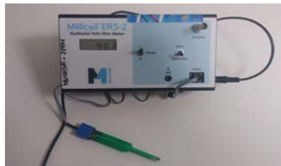
Fig. 2. TEER measurement components
