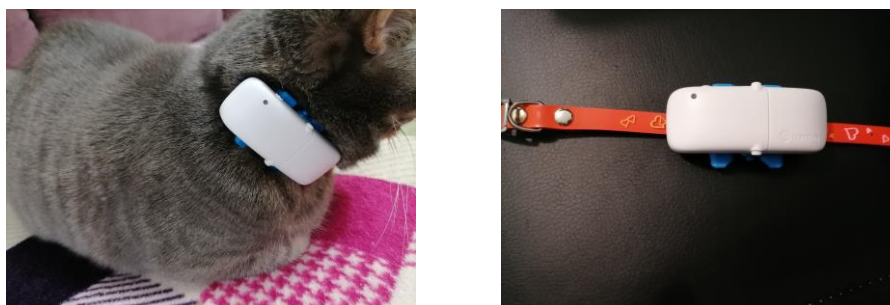
Fig. 1. The Tractive IKATI GPS device attached to the regular collar of the cat (original photos)
