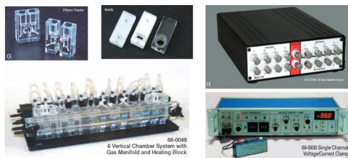
Fig. 2. Components of a Ussing chamber (44)
