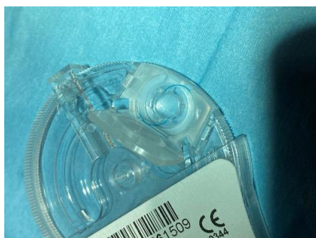
Fig. 9. Soft hydrophobic acrylic IOL with blue PMMA mod C haptic (original photo)
