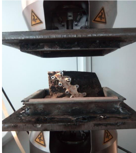
Fig. 3. Testing the resistance of the epoxy material, screw, cerclage in a deep total crack
