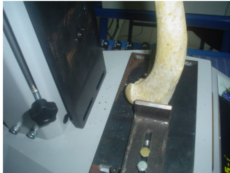
Fig. 2 Humerus, longitudinally stress of the neck
