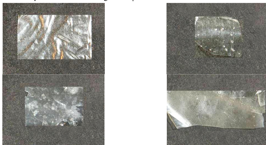
Figure 1. Membranes made of polymers in the following mix ratios: A-100% Col; B-85% Col, 15% PEG; C-50% Col, 50% PEG; D-70% Col, 30% PEG.
